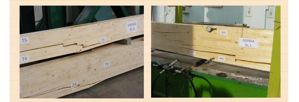
Below you can see the manufacturing technology (the injection of crack using MAPEI Mapewood Gel and the application of carbon fiber tissue MAPEI Mapewrap using MAPEI Mapewood Primer and MAPEI Mapewood Paste)
