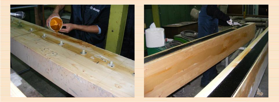
Below you can see the manufacturing technology (the anchorage at the ends and the application of carbon fiber flat band using MAPEI Mapewood Primer and MAPEI Mapewood Paste)
